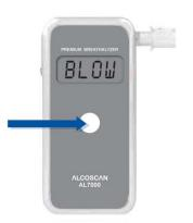
Secure your lips around the mouthpiece and blow sharply and steadily into unit for about 4 seconds.
